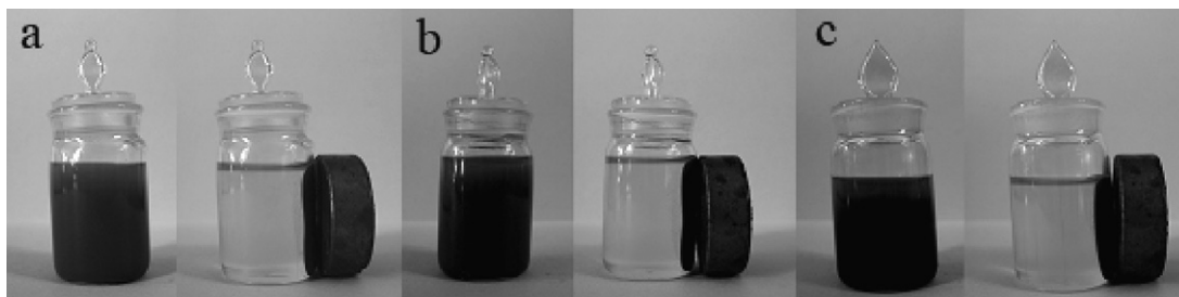
Fig. 7. Illustration of the magnetic separation of MPNSs(MnMP) (a), MPNSs(MnPP) (b) and MPNSs(MnCP) (c) from the liquid media.
